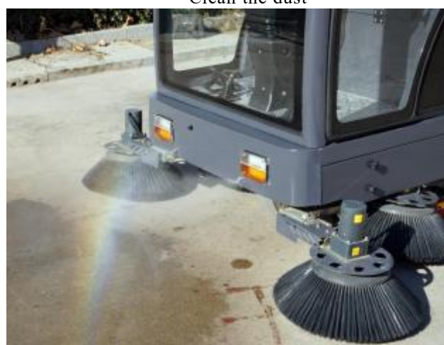
Front-mounted spray system for dust suppression
