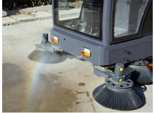
Front-mounted spray system for dust suppression
